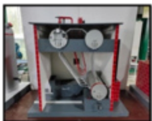
Cut-section Model of Stirling Boiler
