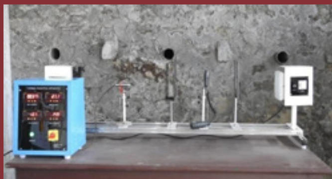
Radiation Apparatus with Radiation Shield Arrangement
